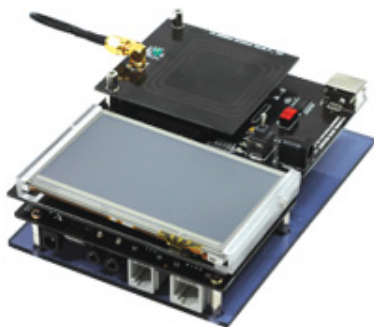
HBE-RF ID-REX (13.56MHz) Example of Using Handheld Reader Types
